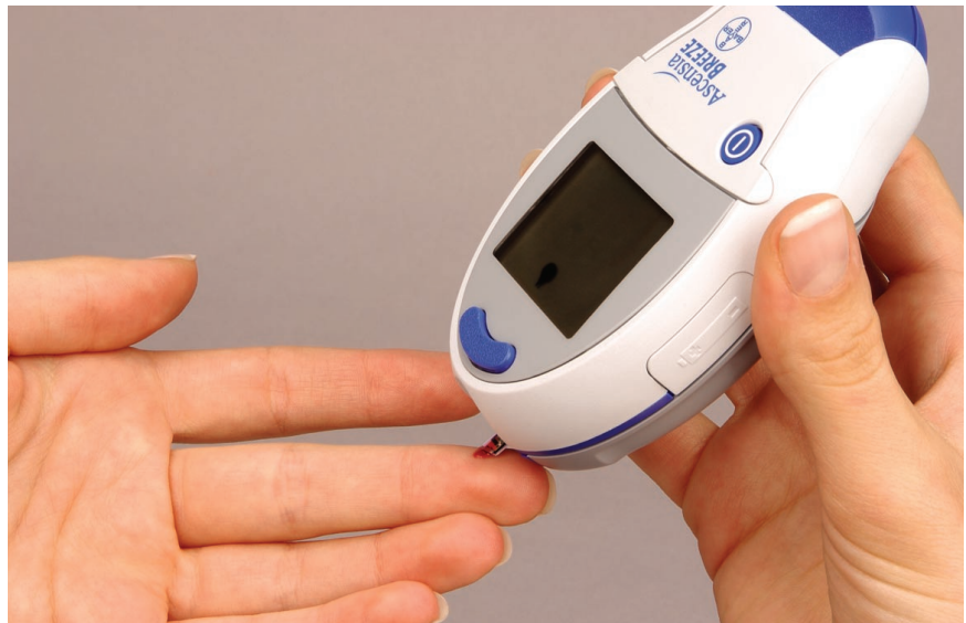
Figure 2. The meter aligned to a finger – the Ascensia Breeze has an indentation at the point where the sensor protrudes from the meter
