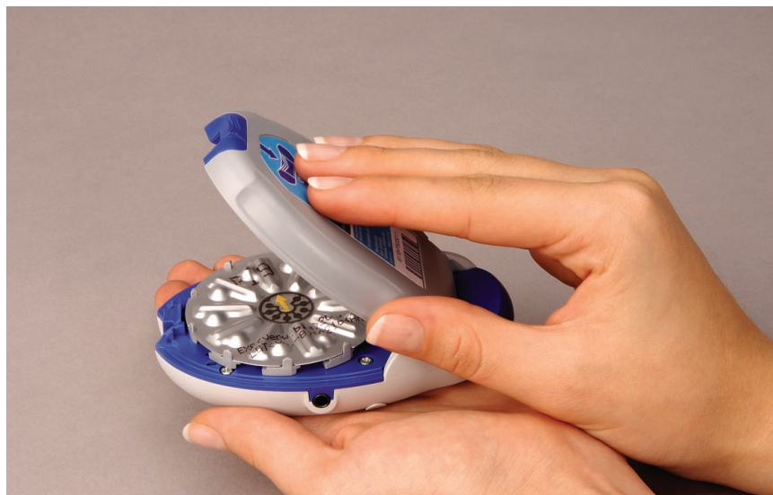
Figure 1. The meter opens with a catch at the sensor end
